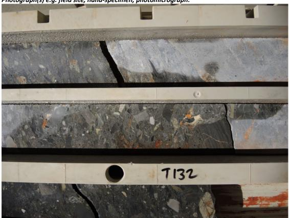
Photograph of typical weakly sericite altered polymict conglomerate from just beneath the sample interval.
